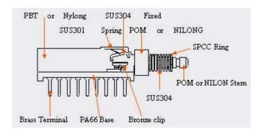
Case: High Temperature PBT or NYLONG (UL94 V-0)
