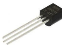
2N2907 TRANSISTOR PNP 0.6A 60V 0.4W TO-92
