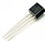
2SA1015 TRANSISTOR PNP 150MA 50V 400MW
