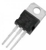
TIP42C TRANSISTOR PNP 6A 100V
