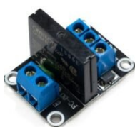
MODSSR1L MOD 1CH SSR 5V 2A LOW LEVEL
