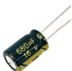
E680X16 CAPACITOR ELEC 680UF 16V 105° 10X13MM HF
