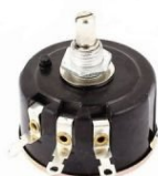
WX112-472 POTENCIOMETRO LINEAL CARBON 5W 4K7 1V
