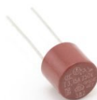
FR2A FUSIBLE RAP RADIAL 8.5X7.2MM 2A 250V
