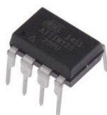
ATTINY25-20PU MICRO 8 BITS 2KB FLASH 0.128KB
