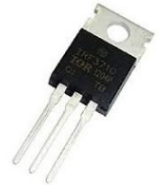
IRF3710 MOSFET N 57A 100V 0.023 OHM 200W TO-220
