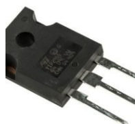
TIP2955 TRANSISTOR PNP 15A 60V 90W TO3P
