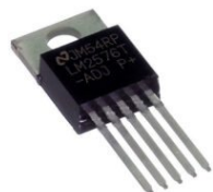
LM2576T-ADJ STEP DOWN AJUSTABLE 3AMP
