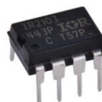
IR2103 HALF BRIDGE DRIVER MOSFET
