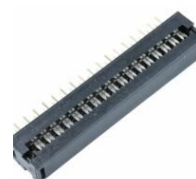
IDC34MC2 CONECTOR IDC 34 VIAS MACHO P/SOLDAR PLACA
