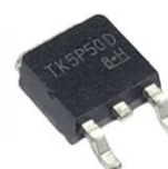
TK5P50D MOSFET N 5A 500V TO-252
